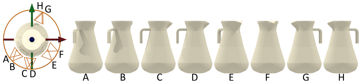
Figure 4.6: Different metrics considered for finding the master camera placement. The viewpoints maximize: (A) Silhouette Curvature Extrema, (B) Silhouette Curvature, (C) Projected Area, (D) Silhouette Length, (E) Surface Visibility, (F) Maximum Depth, (G) Depth Distribution, (H) Viewpoint Entropy. The maximum silhouette length (D) decreases part occlusion.
